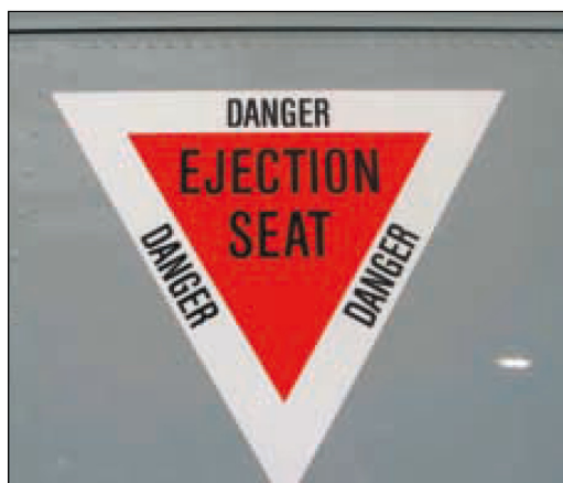
Ejection seat warning on military/ex-military aircraft
