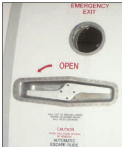
Typical external door handle markings
