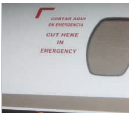
Emergency cutting area on aircraft fuselage
