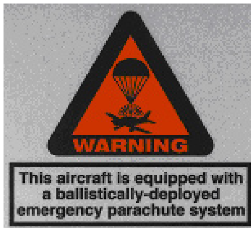
Ballistic recovery system warning sign
