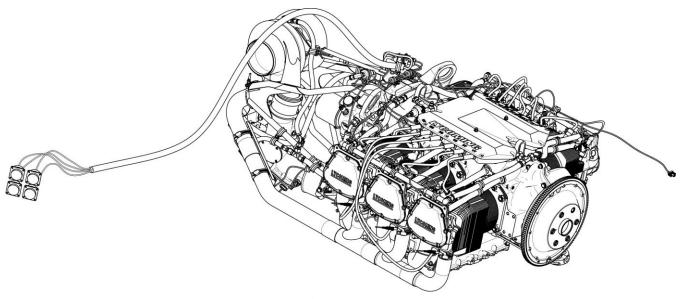
Figure 1 Engine Wiring Harness Installed on TEO-540-C1A Engine
