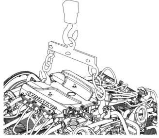
Figure 3 Engine Lift
