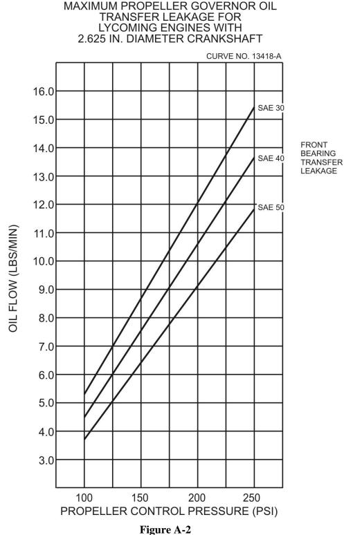
Propeller Governor Oil Transfer Leakage Rate
