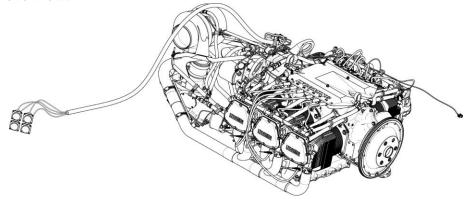
Figure 4 Engine-to-Firewall Wiring Harness
