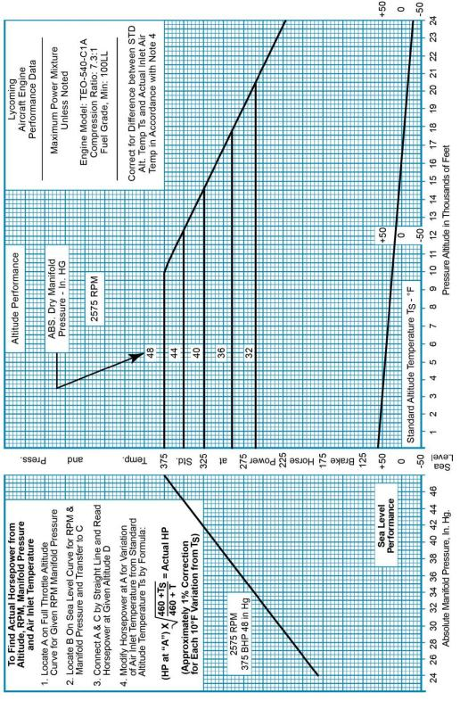
Figure A-3 2575 RPM Sea Level and Altitude Performance
