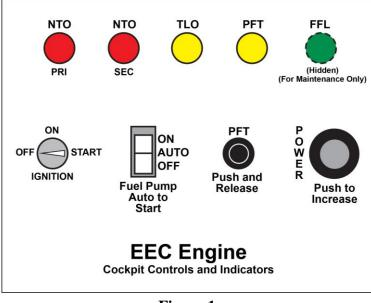
Figure 1 EECS Cockpit Controls and Indicators
