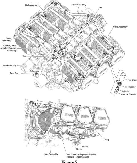
Figure 7 TEO-540-C1A Engine Fuel System
