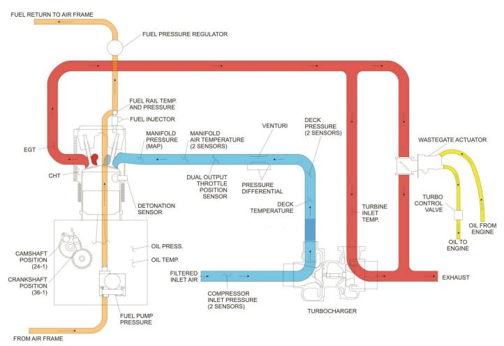
Figure 2 EECS Integrated Controls
