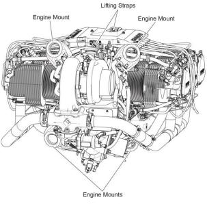
Figure 4 Engine Mounts
