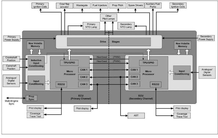
Figure 6 Engine Control
