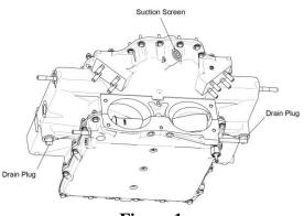
Figure 1 Oil Sump Drain Plugs and Oil Suction Screen
