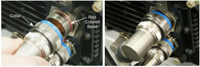
Figure 2 Red Colored Band on the Receptacle
