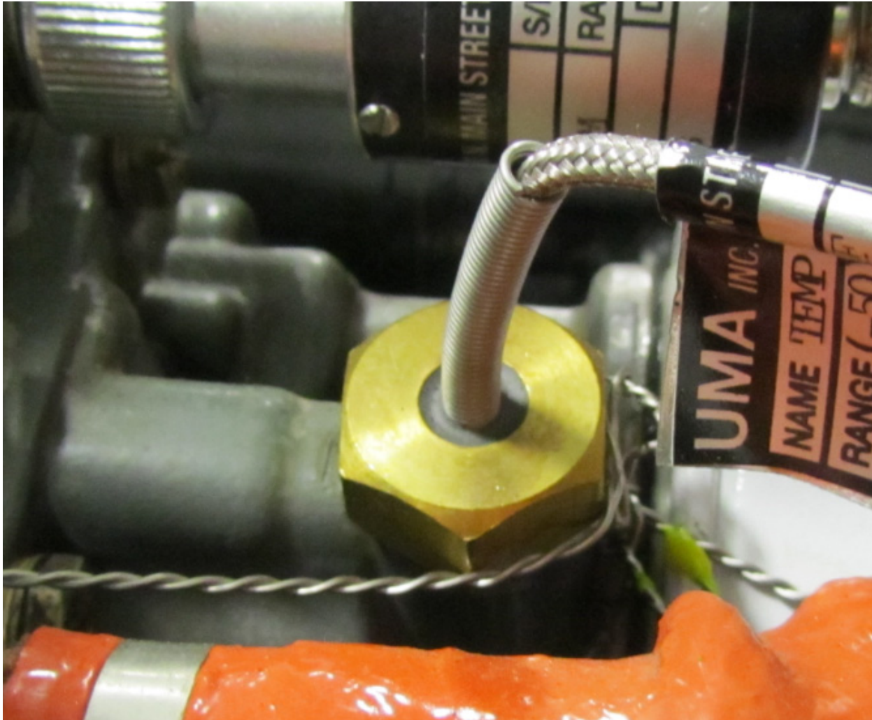
Figure 5-20 Oil Temperature Sensor Installation Example
