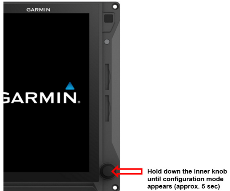
Figure 2-1 Entering the configuration mode on the GDU
