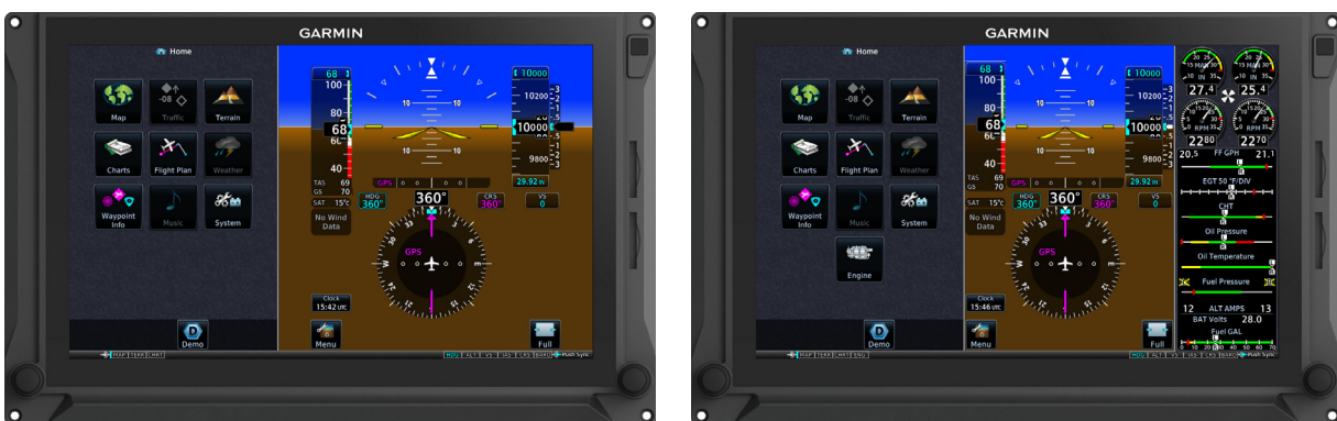
Figure 2-6 The GDU 1060 functioning as an MFD/PFD and MFD/PFD/EIS
