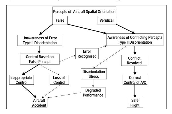
Figure 2. Diagramatic representation of how Type I and Type II spatial disorientation can effect the pilot's control of the aircraft
