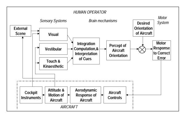
Figure 1, Block diagram of closed-loop, control of aircraft spatial orientation. The pilot receives feedback from vestibular and kinaesthetic receptors, stimulated by angular and linear accelerations, that are phase advanced on the velocity and displacement of visual cues.
