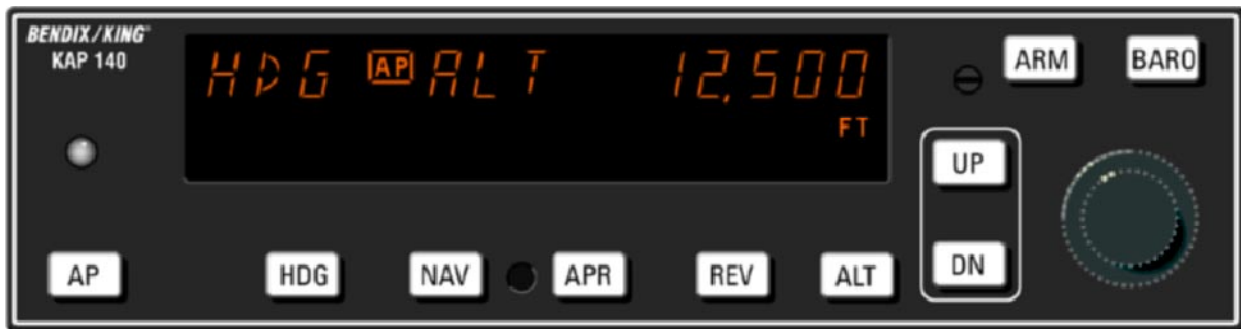
FIGURE 2-3 TWO-AXIS FCC W/ALTITUDE PRESELECT AND ALERTING (-7XXX VERSIONS)
