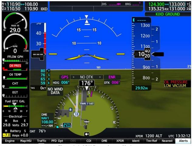
Figure 9-4, GDU Reversionary Mode
