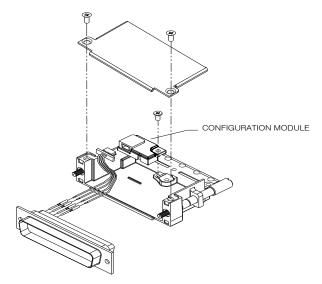
Figure 6-2, GSU 75 Configuration Module Installation
