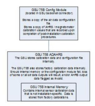
Figure 3-5, GSU Configuration Settings Storage
