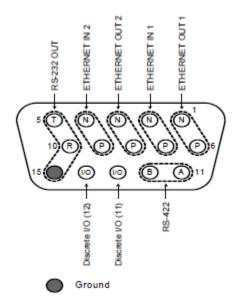
Figure 5-7, GTX 345R (Only) Looking at Front of Connector (P3252)
