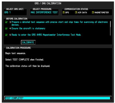
Figure 5-5, Magnetometer Interference Test
