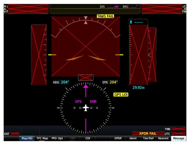
Figure 9-2, PFD Power-up System Annunciations
