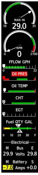
Figure 7-3, Normal Engine Instrument Markings (MFD)
