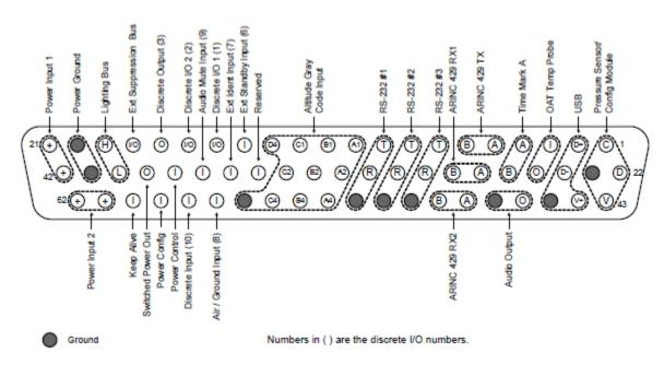
Figure 5-6, GTX 335R/345R Looking at Front of Connector (P3251)
