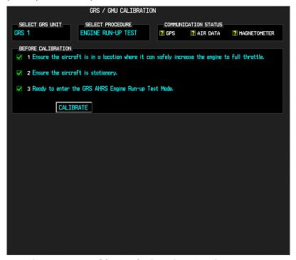
Figure 7-6, GRS/GMU Calibration, Engine Run-Up
