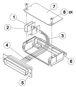
Figure 6-1, Configuration Module Installation
