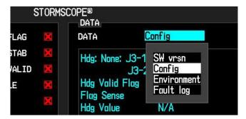
Figure 3-12, Stormscope Configuration
