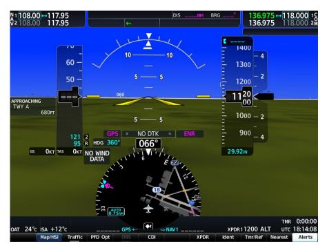
Figure 7-7, Normal Mode AHRS Check
