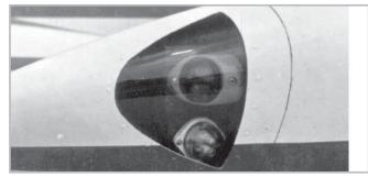
Bend and trim the adapter plate as necessary, so that the A625 clears the transparent window that covers the navigation light area 0.060 inch minimum. The conduit for the navigation light wire is very small. To get the necessary wires to operate the strobe light and the navigation light through this conduit, use a 20 gauge wire, with less that 0.060 inch OD. It has been found that the Belden 8502 or 8308, has an 0.058 inch OD.
