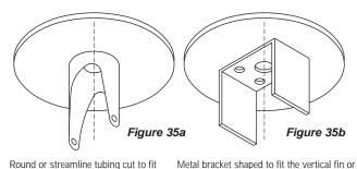
rudder or vertical fin welded to 2 /12" OD rudder with 2 1/2" OD .040" thick disc riveted .40" thick disc. (Reference AC 43.13-1B, in place. (Reference AC 43.13-1B, Chapter 2). Chapter 2, Section 2)
