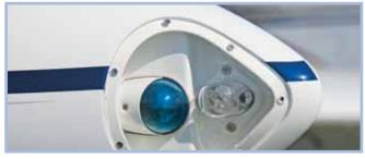
A625 INSTALLATION IN CESSNA 300 OR 400 SERIES WINGTIP TANKS. The A625 fits just under the navigation light, on an adapter plate of 0.032 inch aluminum, approximately 2-3/8 inches x 3-1/2 inches. Fit this plate between the navigation light and its mounting surface, and locate the A625 strobe head below the navigation light.
