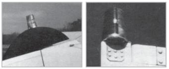
NOTE: Mounting an A450 or A470A strobe lighthead assembly on a vertical fin or rudder, can be accomplished by fabricating a mounting adapter similar to the ones shown in illustrations.
