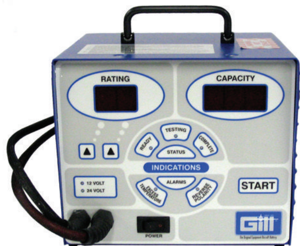
This Gill TCT-1000 battery tester costs well over $1,000. Not too many maintenance shops have one.
