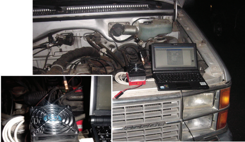
Figure 4 - Using the DBA II to test the capacity of the battery on my old "airport car."
