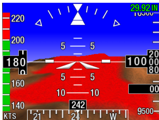
Figure 3-17: Terrain Warning Alert
