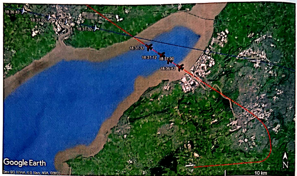
ABOVE: illustration from an ARC report. The crew of an ATR turboprop (red track) had reported to the Airprox Board that they'd encountered a quadcopter drone over the Bristol Channel at FL78. Noting that the possibility of a drone being able to reach this altitude at that location would be unlikely, ARC postulates from ADS-B data that the actual object was a distant A320 seen at the same relative angle
