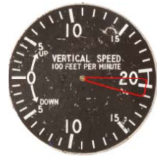
Fig. 7: Vertical Speed. The red triangle indicates 1900 to 2000 ft/min DOWN, the sector where impacts were registered on the instrument.
