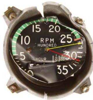
Fig. 6: Rpm Indicator. Needle impacts were detected from 2800 rpm, yellow arrow. The red arrow indicates 3200 rpm, the maximum rpm reached.
