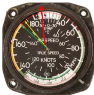
Fig. 5: Airspeed Indicator. The yellow arrow indicates 173 mph, the green arrow 170 mph and the red arrow indicates 188 mph, the maximum airspeed reached.
