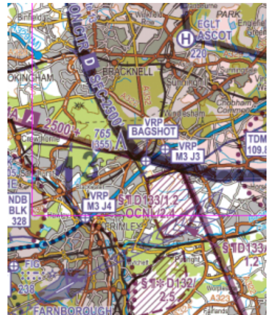
Note the potential for confusion between the Bagshot mast and the Bagshot VRP
