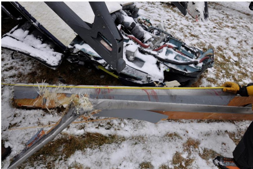
Photo 9: helicopter main rotor blades damages.
