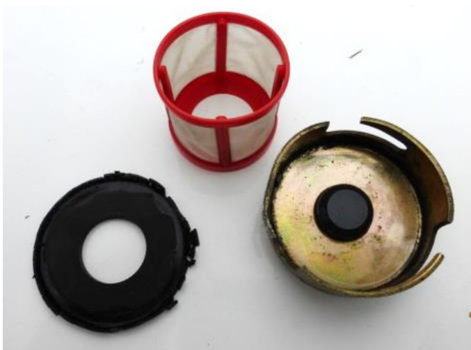
Illustration 4: Strainer of the electric fuel pump with cracked seal
