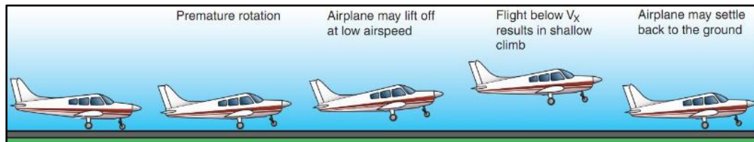
Illustration 3: Take-off at low speed in the ground effect (source: Airplane Flying Handbook FAA-H-8083-3A)
