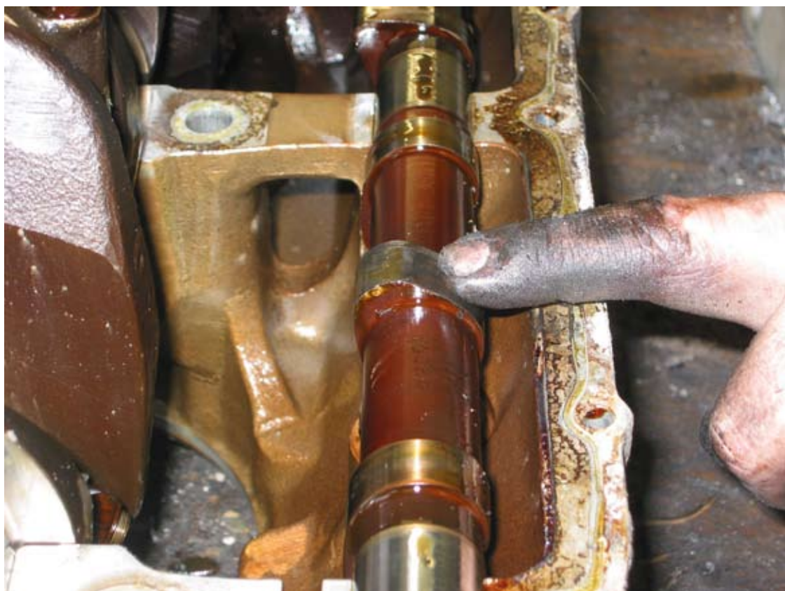
Worn cam lobe, as found during engine strip
