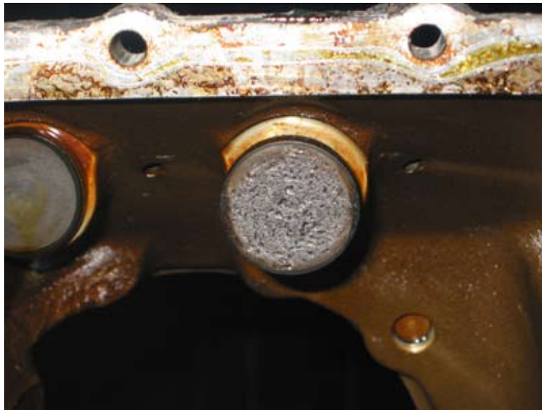
View of spalling on one of the cam followers
