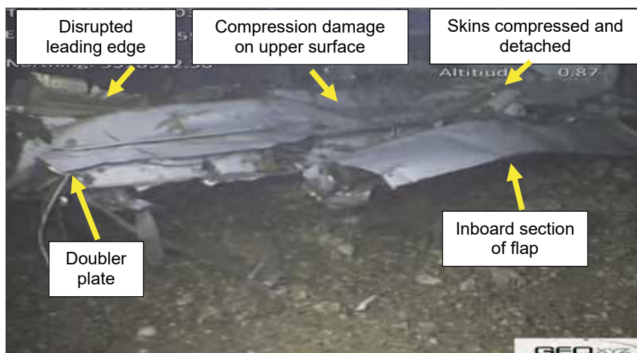
Figure 15 Damage to left wing
