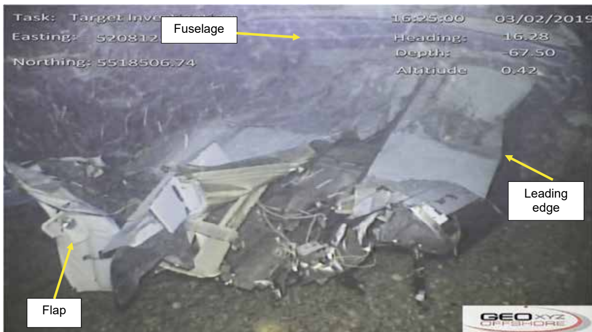
Figure B-8 Remains of right wing
