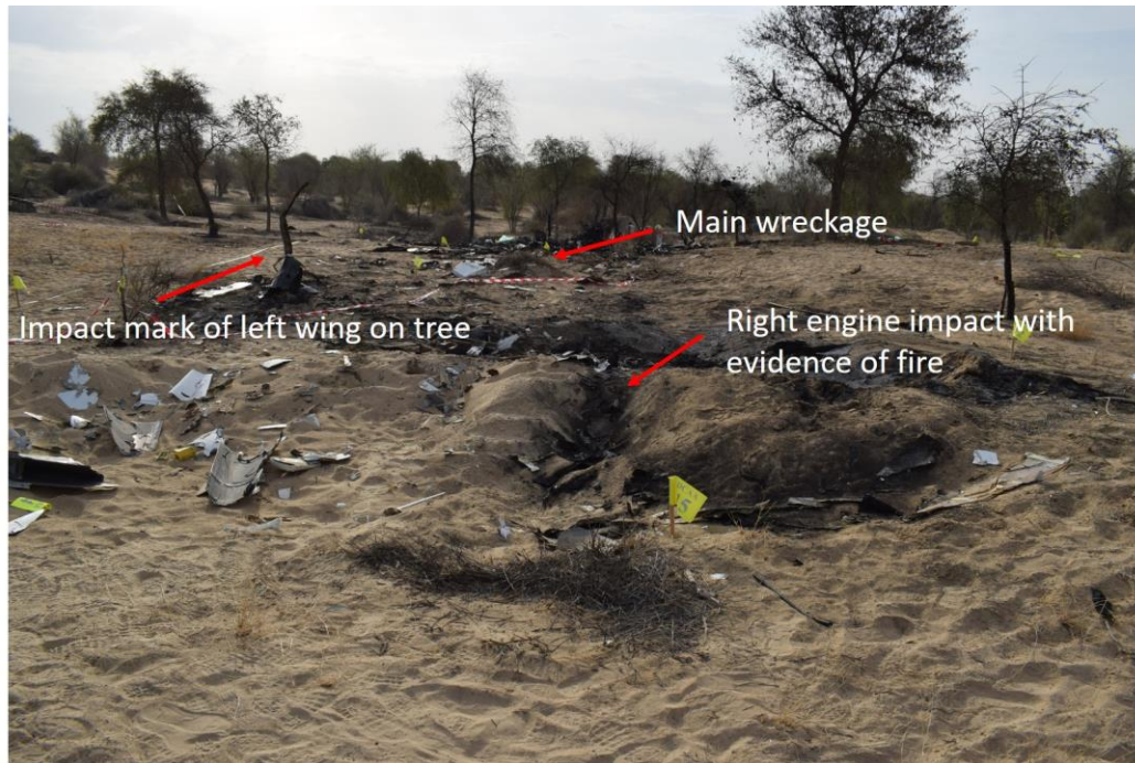
Figure 6. The initial impact point ground scars
