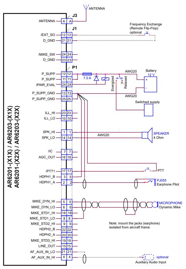
Figure 2-19: Wiring for Single Seat Glider
