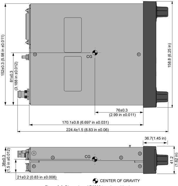
Figure 2-6: Dimensions AR6203 top view, side view
