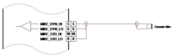
Figure 2-32: Modified Dynamic Microphone Wiring Interface for AR6201
