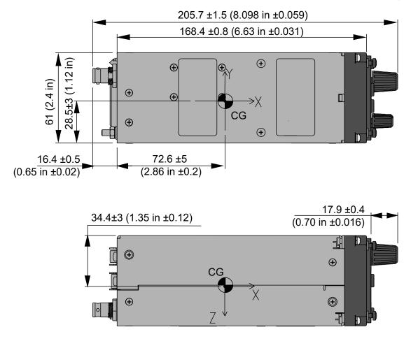
Figure 2-5: Dimensions AR6201 (top-, side view)
