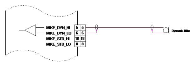
Figure 2-31: AR6201 with Wiring Interface for AR4201
