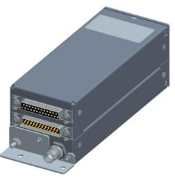
Figure 1-3: RT6201 Remote Transceiver
