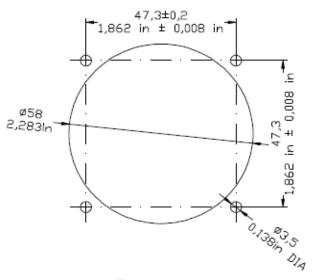
Figure 2-3: Drilling template (back panel mounting)
