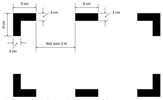
(2) The colour of the markings must be red or yellow and, if necessary, must be outlined in white to contrast with the background.
