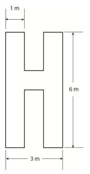
indicates an area which must be used only for the taking off and landing of helicopters.
