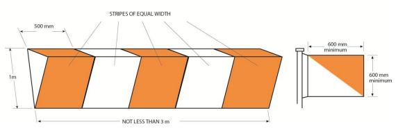
indicate the boundary of an area unfit for the movement of aircraft.
