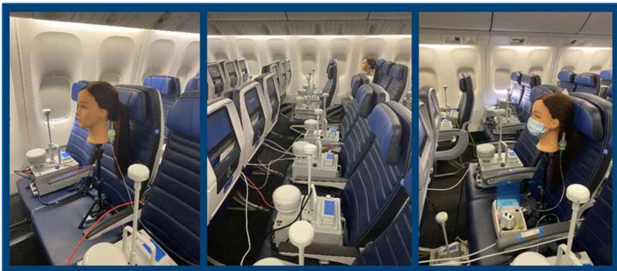
Figure 1: IBAC sensors with extended inlets and tripod mounted mannequin with integrated aerosol generation
