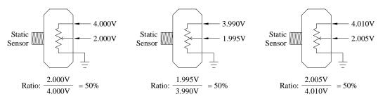
Figure 1 Ratiometric ratio stays the same if voltage supply varies.
