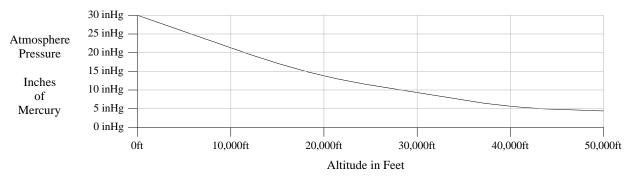
Figure 3 Altitude and atmospheric density relationship.
