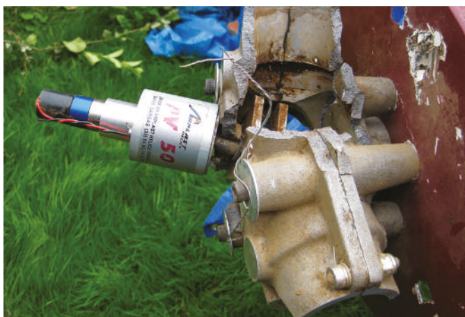
Above In 2007, the pilot of a Europa suffered a loss of propeller thrust shortly after take-off, and in 2018, the pilot of a Kitfox Mk. 7 lost propeller thrust whilst at altitude. Both aircraft were substantially damaged during the following forced landing. In both cases, the initial cause of the propeller pitch mechanism failing was found to be a 'stripped' leadscrew. Photos: Malcolm McBride/ Alan Bray
