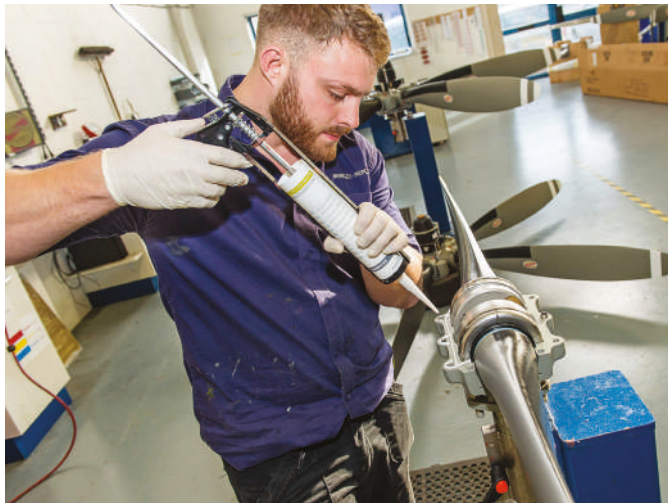
Above An LPIP inspection takes into account that a propeller that hasn't completed many hours will not need specific checks related to wear and fatigue, so there's not a requirement to strip the coatings from blades or carry out expensive non-destructive testing. Photo: Ed Hicks
