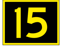
Runway Location Sign
