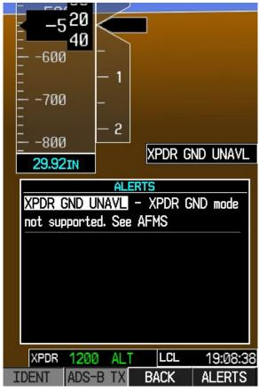
Figure 1-3 XPDR GND UNAVL Annunciation Display
