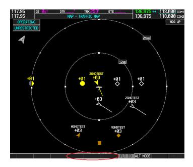
Figure 2-1 Display with ADS-B and TAS/TCAS
