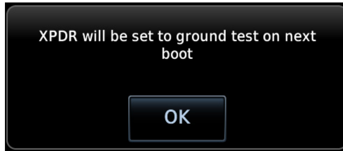
Figure 7-23 XPDR Ground Test Mode Acknowledgment
