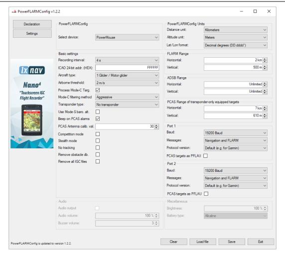
Here you can set all settings for your PowerMouse device. File will be saved as flarmcfg.txt file, which you should save on the USD memory stick. To load this file into PowerMouse, insert USB key into USB slot on PowerMouse and switch on PowerMouse. File will be automatically loaded into device.
