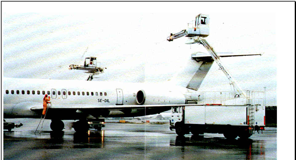
Fig. 6.7) Example of ground ice treatment
