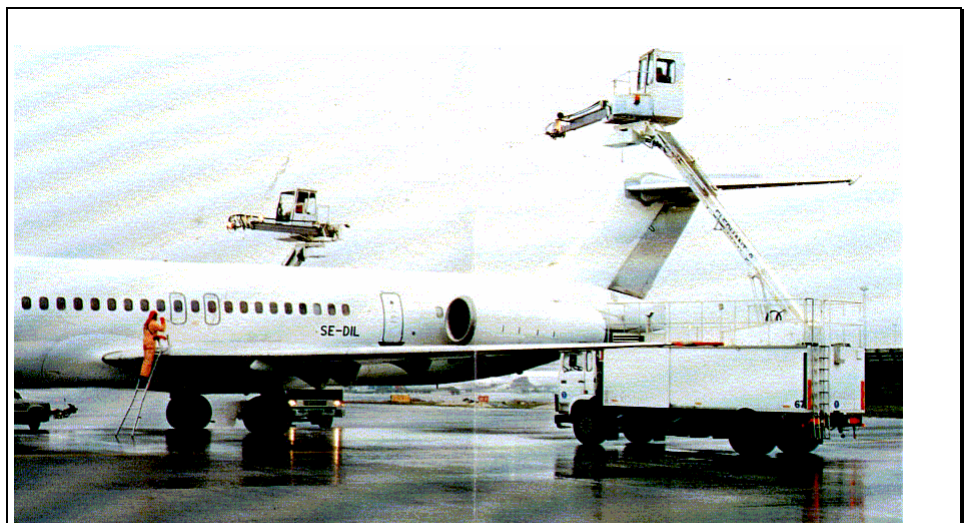
Fig. 16) Example of ground de/anti-icing treatment
