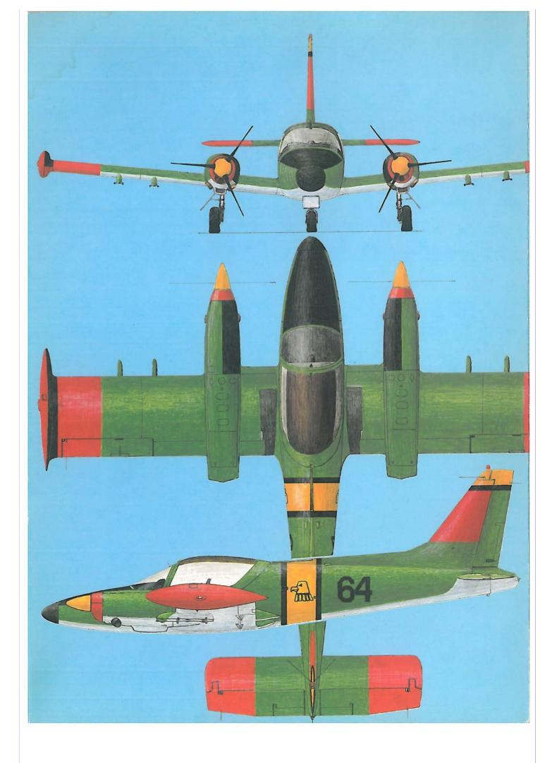
Power Plant: two 420 shp (313 kW) Allison 250-B17C turboprop engines, each driving a Hartzell HC-B3TF-7A/T10173-25/R three-blade propeller.
