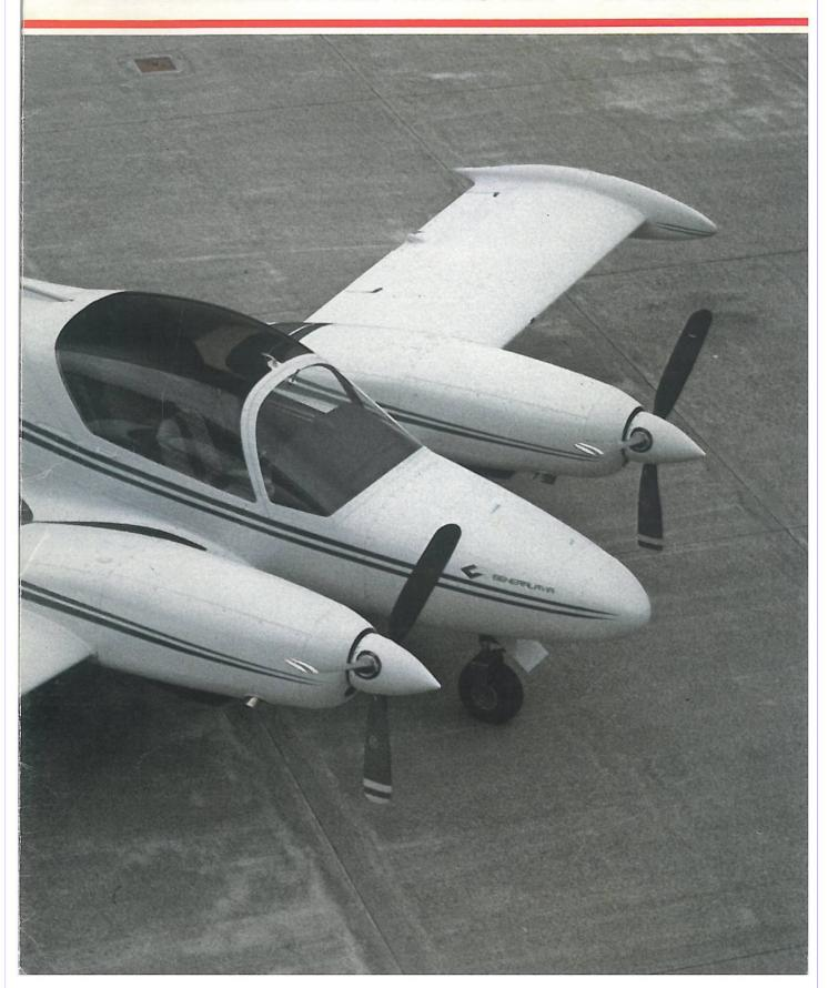
The F.20TP Condor is an all-metal four-seater equipped with two highly reliable turboprop engines, for a total output of 840 shp.
