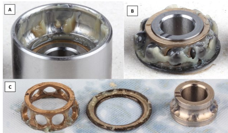
Bearing in new condition - (A) Housing and outer race, (B) inner race, cage and balls assembled, (C) cage, seal and inner race disassembled
